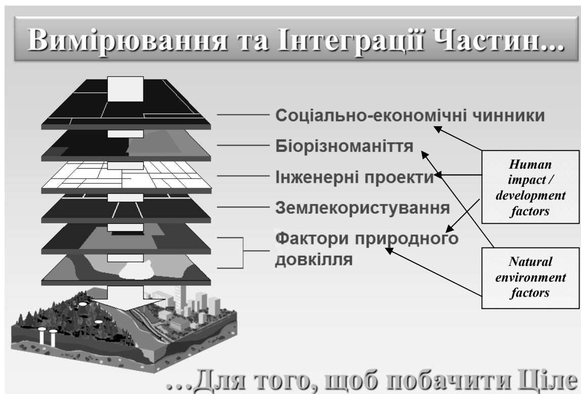
Fig. 2. Strategic goal of the environmental geography: human / natural environment data integration with further visualization through GIS. The layers sequence is presented according to the accepted GIS rules
