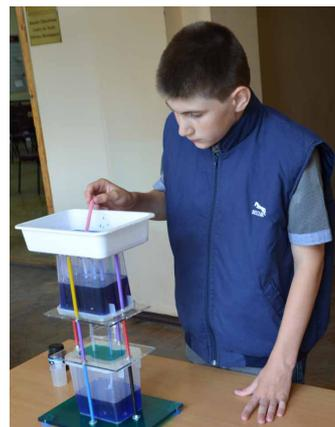
Fig. 2. Working with real tools and the example of hands-on Heron Fountain from the plastic boxes as a second stage project
