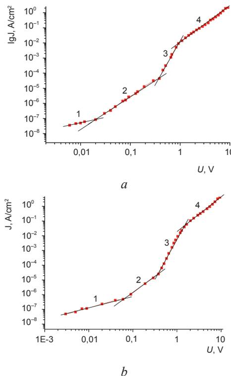
Fig. 2. Direct branch of the CVC for typical Schottky diodes (Al-p-CdTe-Mo) in double logarithmic scale in the dark at  $T = 300$  K. The area of Al-contact  $S \approx 0.07$   $\text{cm}^2$ , ( $a - w = 8$   $\mu\text{m}$ ,  $\rho \approx 2 \cdot 10^8$   $\Omega \cdot \text{cm}$ , base — sample No. 1,  $b - w = 10$   $\mu\text{m}$ ,  $\rho \approx 2 \cdot 10^7$   $\Omega \cdot \text{cm}$ , base — sample No. 2)
