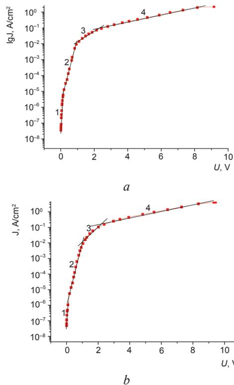
Fig. 1. Direct branch of the CVC for typical Schottky barrier diodes (Al-p-CdTe-Mo) in semi-log scale in the dark at  $T = 300$  K. The area of Al-contact  $S \approx 0.07$   $\text{cm}^2$ , ( $a - w = 8$   $\mu\text{m}$ ,  $\rho \approx 2 \cdot 10^8$   $\Omega \cdot \text{cm}$ , base — sample No. 1,  $b - w = 10$   $\mu\text{m}$ ,  $\rho \approx 2 \cdot 10^7$   $\Omega \cdot \text{cm}$ , base — sample No. 2)
