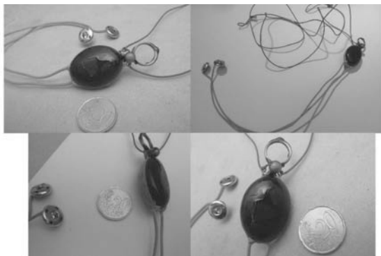
Figure 2. Multiple views of the final ECG sensor
