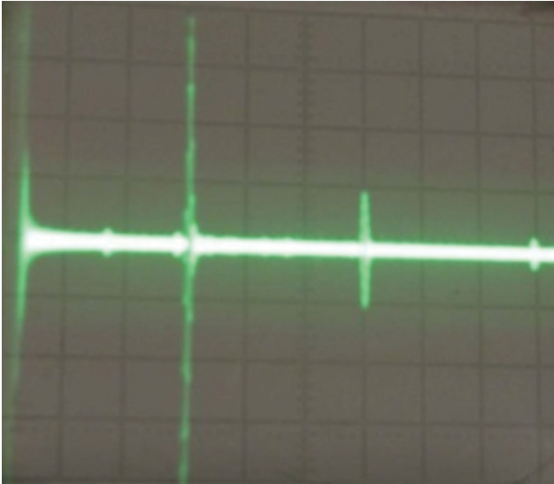
Fig.5. Time sweep with the received signal, obtained using EMAT presented on Fig.3 (vertically - 10 mV / div, horizontally 10 \mu s)
