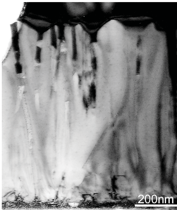
Fig. 2.8. Typical structure of GaN layers after annealing in Zn vapor at temperature of 1200°C.
