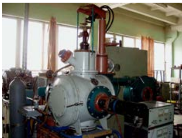
Fig. 1 Installation "Strychka" for fabrication of metal films with a complicated nonequilibrium structure.
