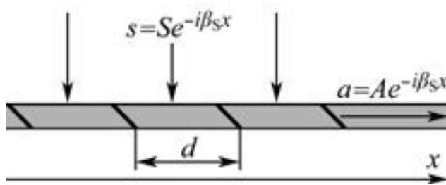
Fig.3. The scheme of spatial connection of the wave  $s$  incident on the waveguide (gray bar) with waveguide mode  $a$  through the grating with spatial frequency  $\beta_s = 2\pi/d$ . SG strokes are black oblique lines in the waveguide.
