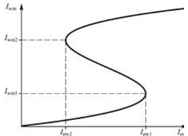
Fig.4. The qualitative form of the intensity of the waveguide mode  $I_{wm}$  on the intensity of the pump wave (laser beam)  $I_{pw}$  obtained from the equation (7).
