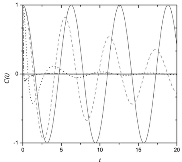
Fig. 2. The  $C(t)$  dependence of the normalized correlation function of the Langevin force at different values of the parameter  $\alpha = \gamma k_B T / M\omega_0^2$  ( $\alpha = 0.1$ , dashed line;  $\alpha = 1$ , dotted line;  $\alpha = 10$ , dash-dotted line; the case of linear oscillations corresponds to  $\alpha = 0$ , solid line).
