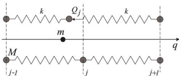
Fig. 3. Model of 1D lattice with longitudinal displacements.
