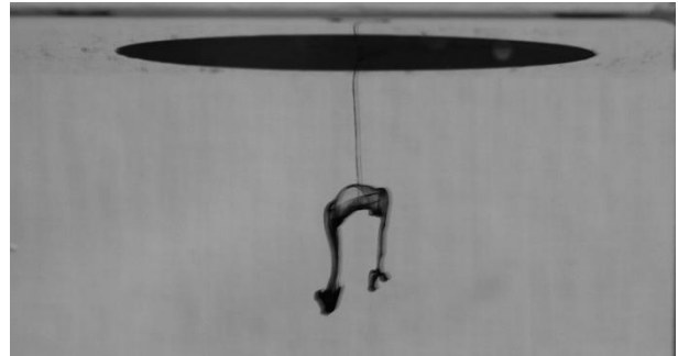
Fig. 1: Spreading and dissolving a droplet of aniline ink deposited to the surface of distilled water.
