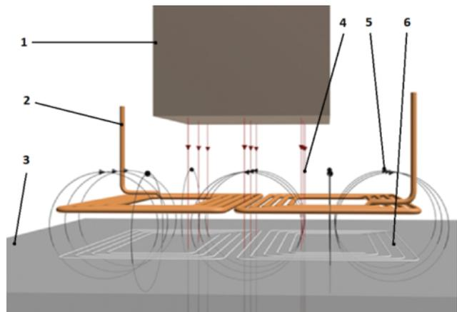
Fig.3. Schematic design of the EMAT, allowing to excite and receive pulses of volumetric shear ultra-sonic vibrations in an electrically conductive ferro-magnetic product.
