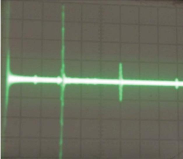
*Fig.5.* Time sweep with the received signal, obtained using EMAT presented on Fig.3 (vertically - 10 mV / div, horizontally 10 μs)
