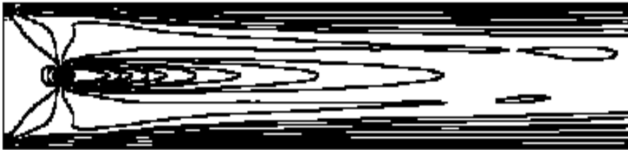
Fig. 4. The lines of equal velocities in the flow around circular cylinder at the Reynolds number Re = 40 , received with LBM
