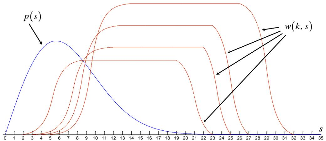
Fig. 2. An example of wind statistics superimposed on PCs (some potential power is cut off)
