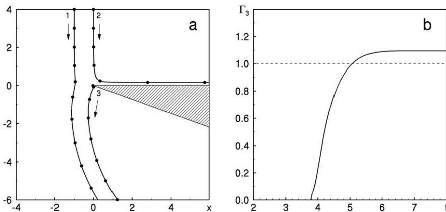
Fig.7. Interaction of the vortex pair with a wedge,  $x_0 = -0.5$ :
