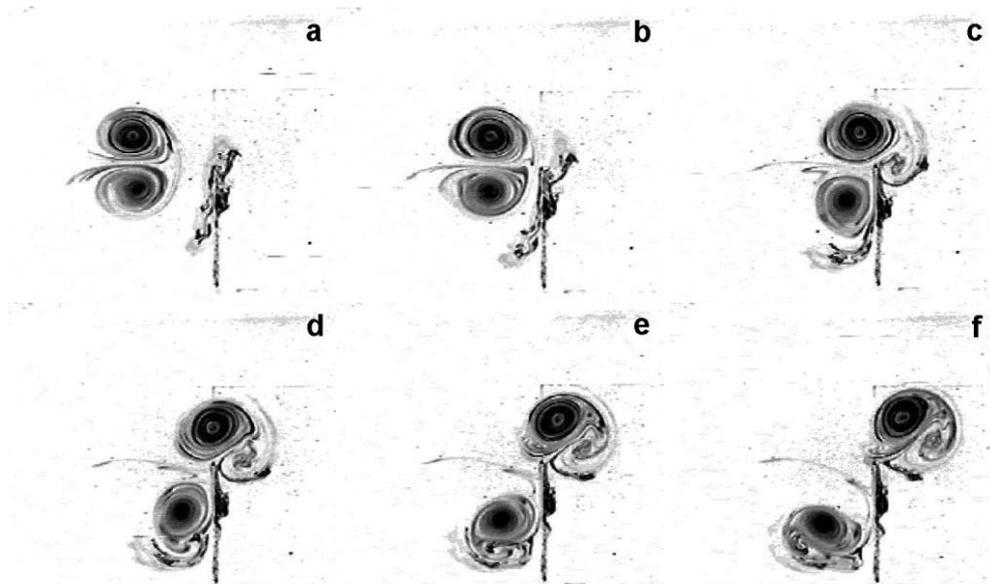
*Fig.4. Dye-visualisation of a dipolar vortex colliding against a flat plate with a sharp edge, with off-set*
