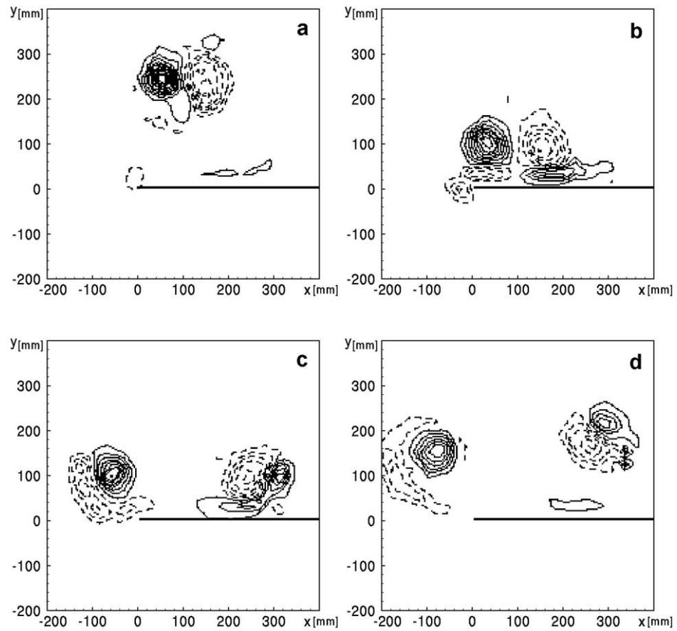
Fig.14. Interaction of the dipolar vortex with a wedge,  $x_0 = 1.0$  (experiment) at:
