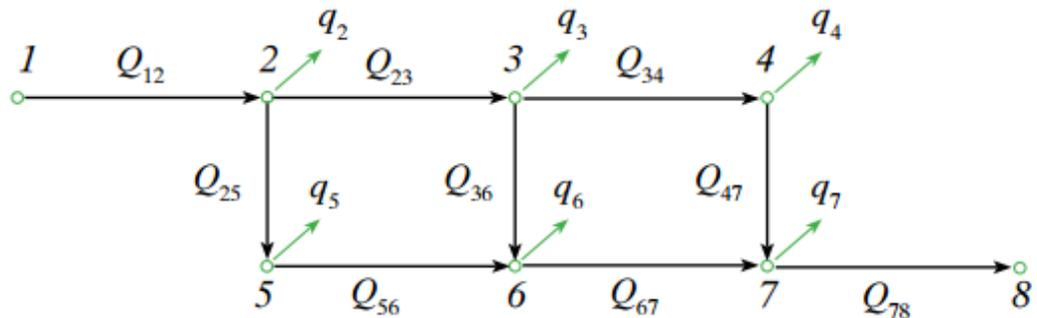
Fig. 2. The principle of naming the hydraulic network graph elements
