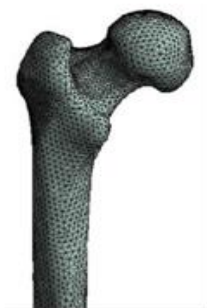
Fig. 9. Finite element model of femur generated by ANSYS [4]
