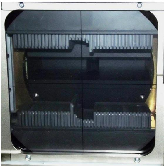
Fig. 7. Multileaf collimator (MLC)
