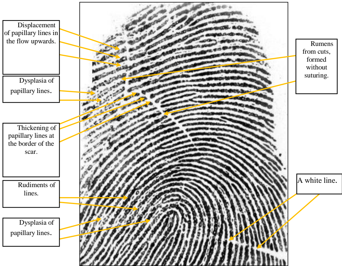
Figure 10. Imprint of the papillary pattern from the nail phalanx of the finger, obtained by using an optical scanner.
