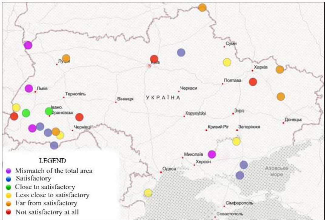
Fig. 6 – Map of the spatial location of NPPs with different levels of compliance with zoning requirements according to DBN B.2.2-12:2019
