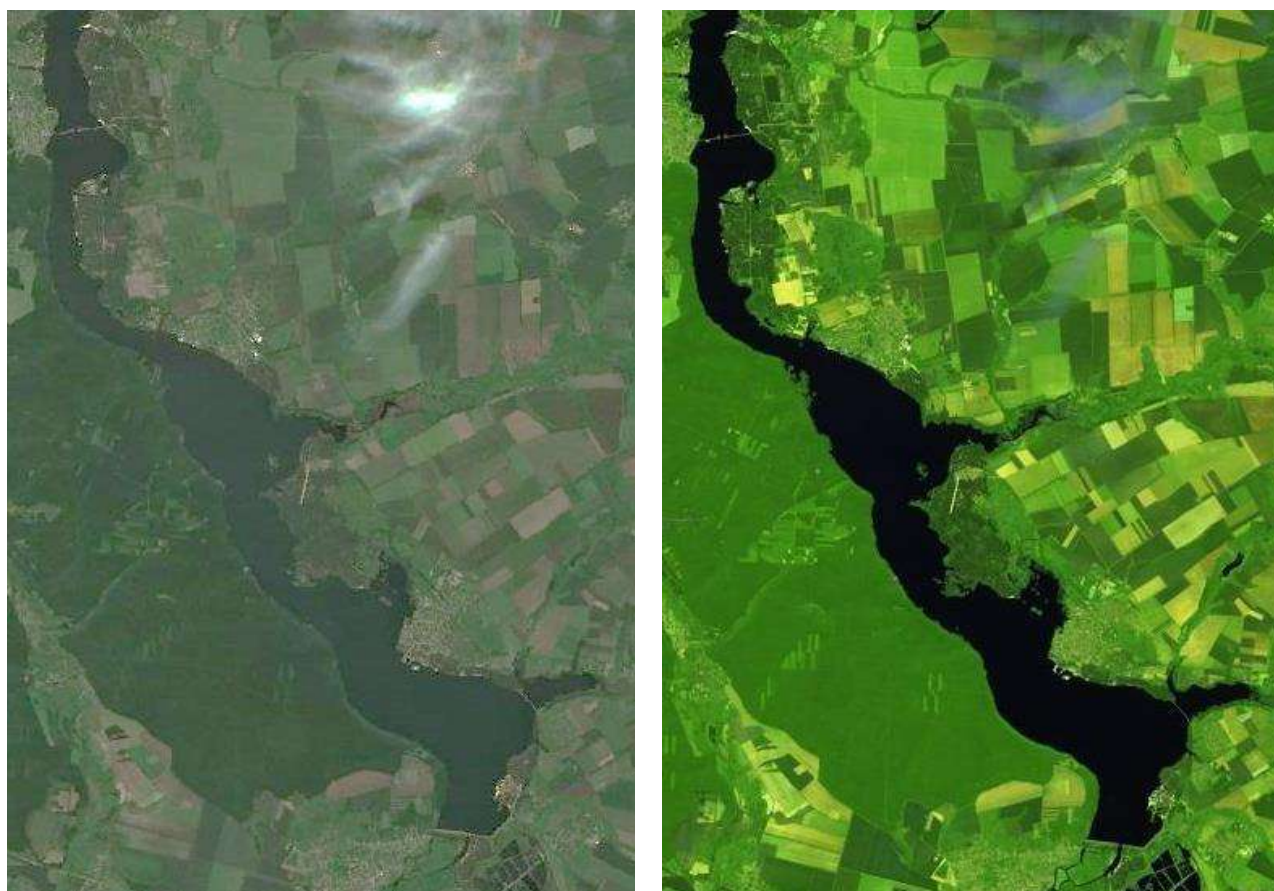
Fig.4. Satellite images of the Pechenihy reservoir. The first one is a composite of natural colors (True Color). The second one is presented in a composite of artificial colors (False Color). Scale 1:400 000 [2]
