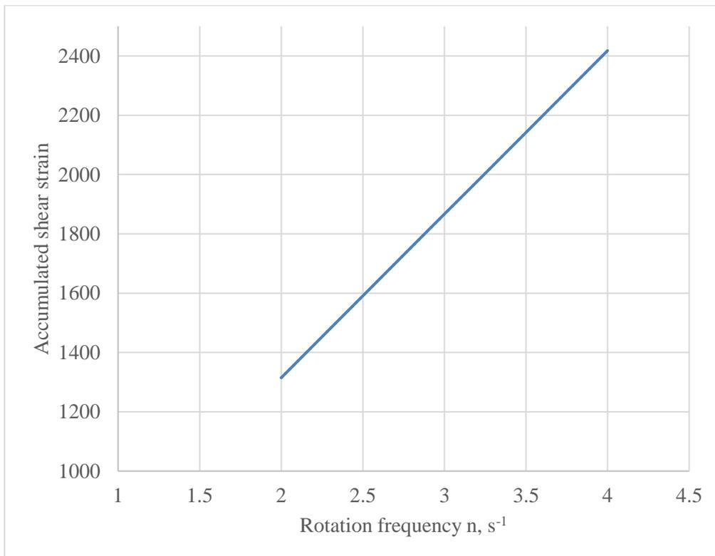
**Fig. 9** - Graph of the dependence of the accumulated shear strain on the working body rotation frequency.
