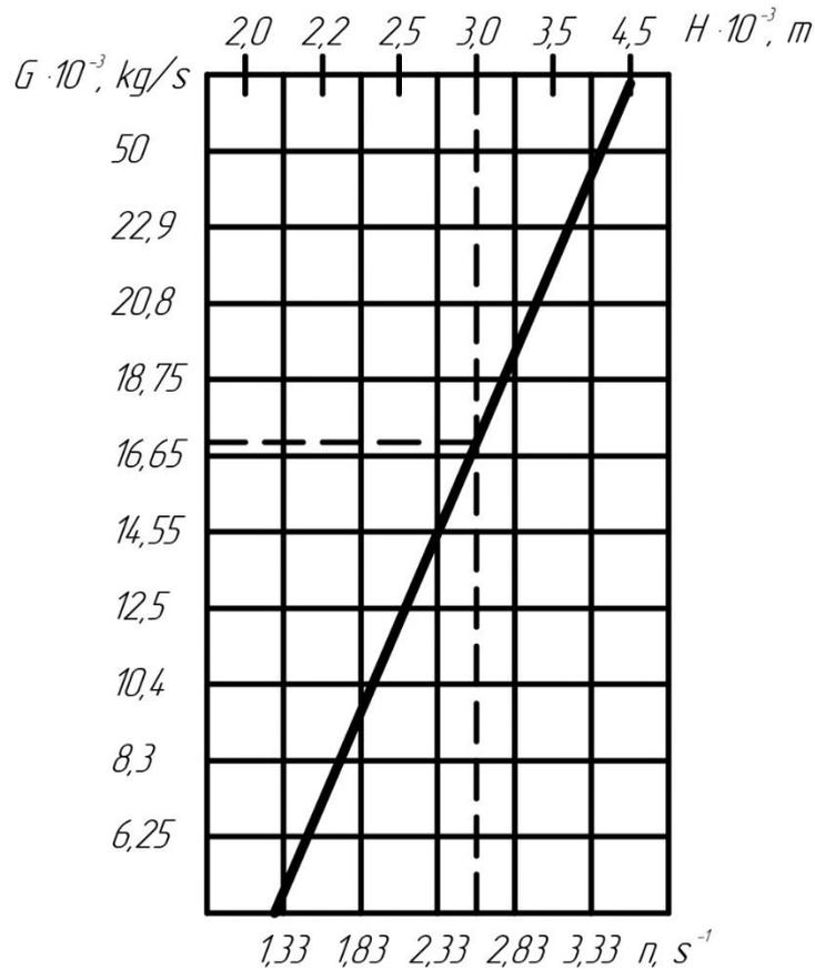
**Fig. 7** - Nomogram for determining the optimal technological parameters of a two-gap disk extruder for processing LDPE of the 15802-020 brand.
