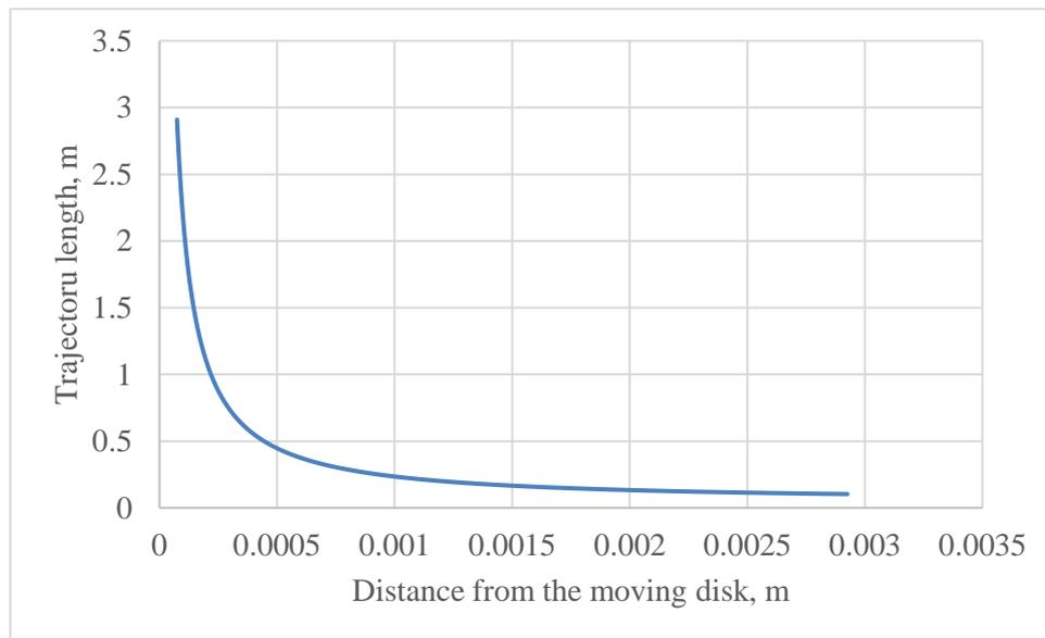
**Fig. 4** - Graph of the dependence of the length of the particle trajectory on the distance from the moving disk when moving in the disk gap of a worm-disk extruder at  $R = 0,065m$ ,  $r = 0,005m$ ,  $W = 7,928 \cdot 10^{-6} m^3/s$ ,
