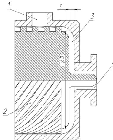
Fig. 1 - Schematic diagram of a disk extruder: 1 - inlet, 2 - screw thread, 3 - disk gap, 4 - outlet.
