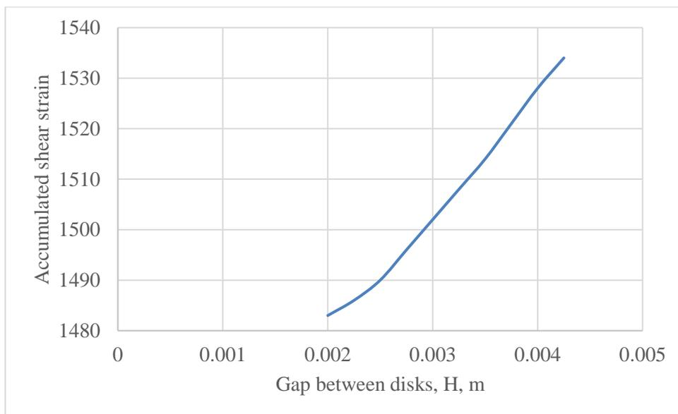
**Fig. 8** - Graph of the accumulated shear strain versus the gap between the disks.**Table 3**
