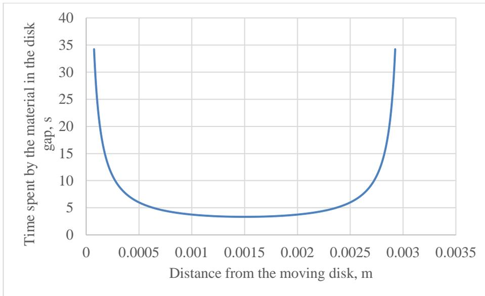
**Fig. 5** - Graph of the dependence of the time spent by the material in the disk gap on the distance from the moving disk when moving in the disk gap of a worm-disk extruder at  $R = 0,065m$  ,  $r = 0,005m$  ,
