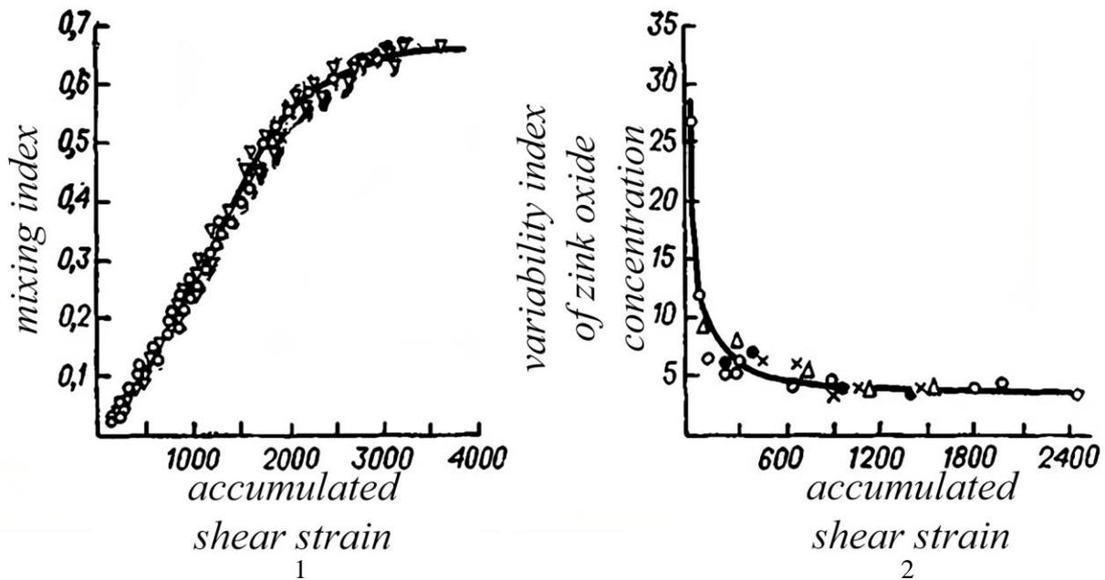
Fig. 2 - The effect of shear strain on the mixing index of polymer mixtures obtained using roller machines (1) and rotary mixers (2)
