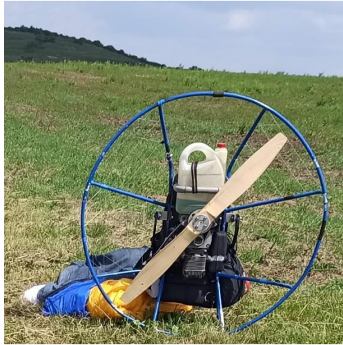
Fig. 3- Exterior view of a paramotor unit with a propeller 125×57 cm
