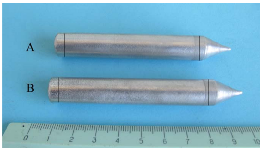
Figure 1. External view of single crystals of cadmium A and B with marked places of cutting samples for research
