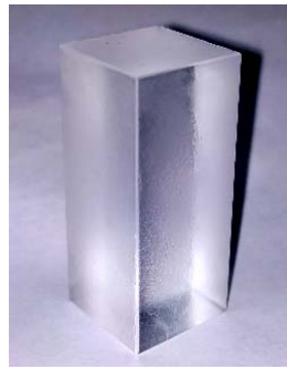
Figure 1. The KDP: TL + crystal sample was grown from water solution.
