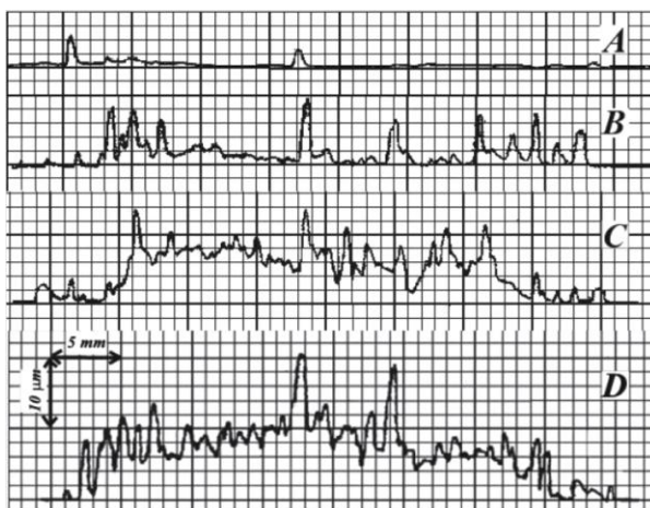
Fig. 11. Evolution of surface profiles of preheated tungsten in the course of plasma exposures. A - 80 pulses, B - 150 pulses, C - 210 pulses, D - 350 pulses
