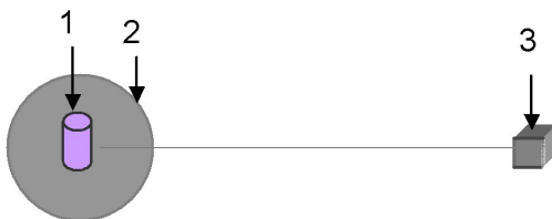
Fig.4. Arrangement scheme of facility elements in the second series of virtual experiments: 1 is neutron source; 2 is a lead sphere; 3 is detector
