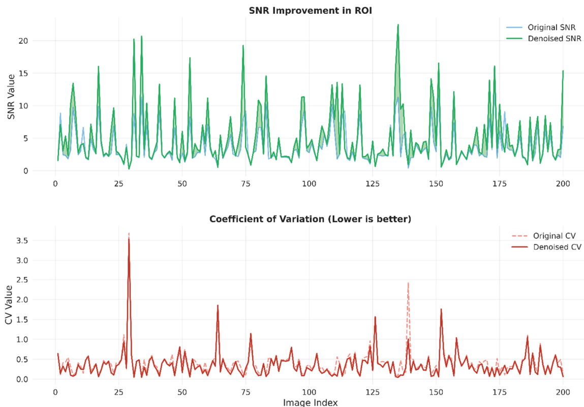
Figure 4. Comparison of Signal-to-Noise Ratio values in homogeneous regions of interest in clinical MRI images before and after noise reduction.
