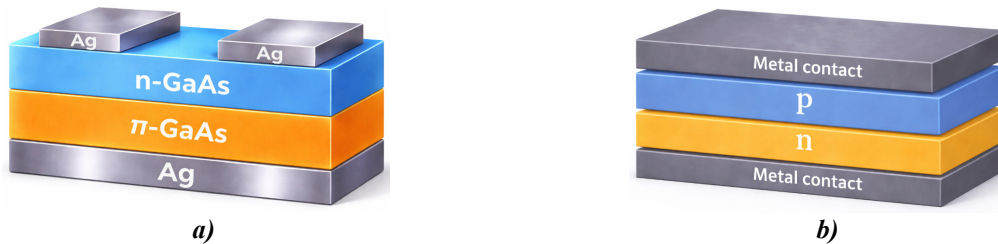
Figure 1. Structural concept and electrical measurement configuration of the fabricated triple-barrier m - p - n - m GaAs-based structures: (a) layered schematic representation of the vertical architecture, and (b) planar cross-sectional view illustrating the coupled metal-semiconductor and p-n junctions.
