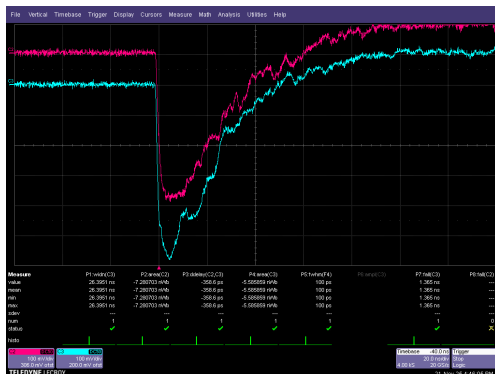
Figure 3. Pulses from coincident events from Na-22 isotope. Corresponding left and right channels, 20GS/s, full bandwidth 3GHz. Baseline noise 2mV avg.
