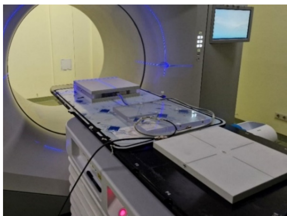
Figure 3. Photograph of measurement setup on TrueBeam with phantom and ionization chamber in position.
