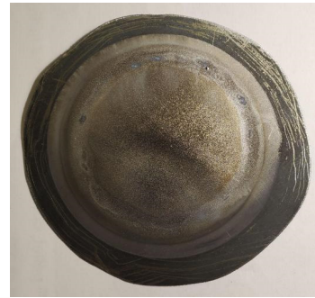
Figure 4. Electron beam imprint on the surface of a molybdenum converter
