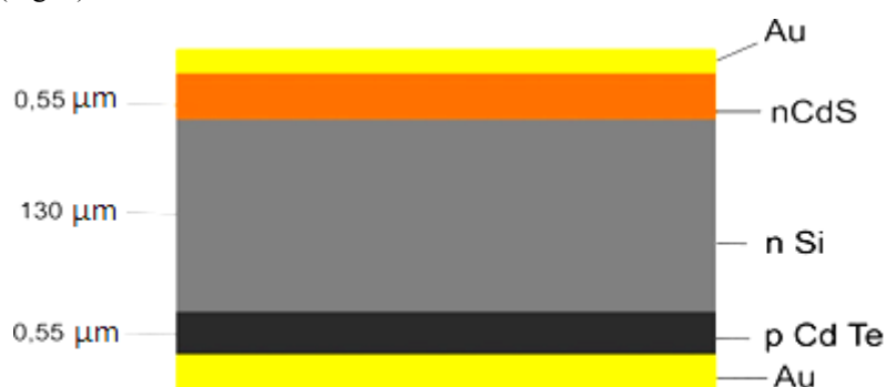
Figure 1. Cross section of a photosensitive multilayer double heterostructure Au-nCdS-nSi-pCdTe-Au
