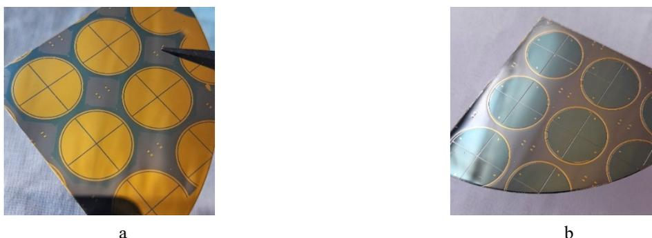
**Figure 1.** Images of silicon wafers at different stages of PD manufacturing: a) after photolithography to open windows corresponding to the gaps between the REs; b) after chemical-dynamic polishing and photolithography to form Au-contact pads.
