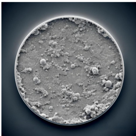
Figure 3. SEM images of n-ZnO grown on sapphire with the scale bar is 2 μm in each figure.
