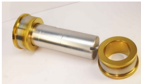
Figure 8. Images of parts ("Axis" - in the center and "Insert" - on the edges) of the friction pair included in the steam distribution unit of the K-325 turbine.
