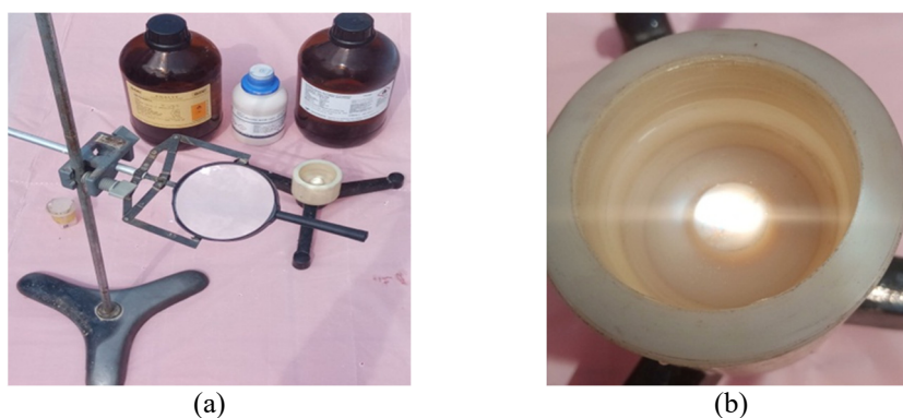
Figure 1: (a) The setup of the system for preparing nanoporous silicon samples, (b) the Teflon container
