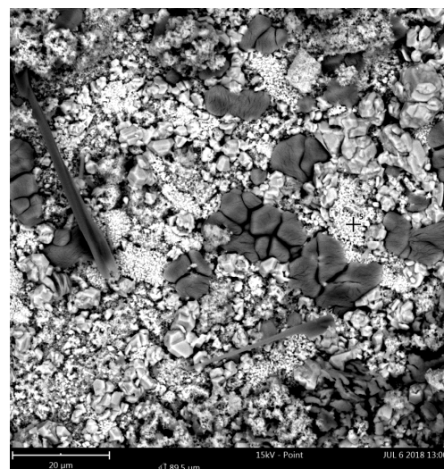
Figure 4. SEM image of CZTS thin film (deposition time of Sn is 5 minute)
