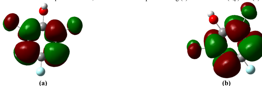
Figure 3. Atomic orbital LUMO compositions for 2,6-dichloro-4-fluoro phenol using (a) DFT/6-311+G(d,p) and (b) HF/ 6-311+G(d,p)
