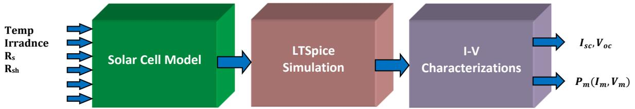
Figure 5. Illustrative diagrams of the inputs and outputs of the LTSpice model.
