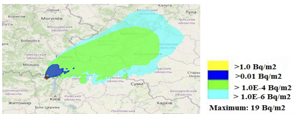
Figure 7. The surface activity of Pu isotopes during deposition on the soil on April 9, 2020 from a fire in the area with Kopachi village - Chistogalovka village (for 24 hours), the source height is 20 m
