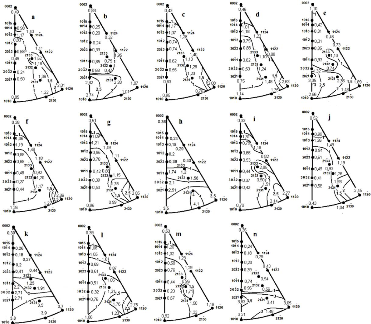
**Figure 1.** Experimental IPFs of the alloy ZE10: (a, b) are IPFs of the original sheet; (c - e) are IPFs after 0.5 of the RB cycle; (f - h) are IPFs after 1 of the RB cycle; (i - k) are IPFs after 3 of the RB cycles; (l - n) are IPFs after 5 of the RB cycles; (a, c, f, i, l) are IPFs of ND; (b, e, h, k, n) are IPFs of RD; (d, g, i, m) correspond to the stretched out sides of the sheets; (c, e, h, l) correspond to the compressed sides of the sheets
