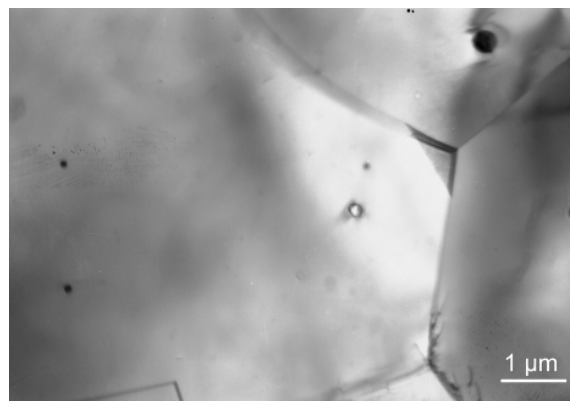
Fig. 1. The initial microstructure of SS316 steel after heat treatment at 1340 K/1 hour.
