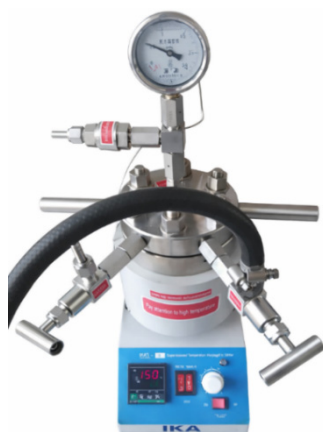
Figure 1. High-temperature sealed reactor for hydrogenation processes
