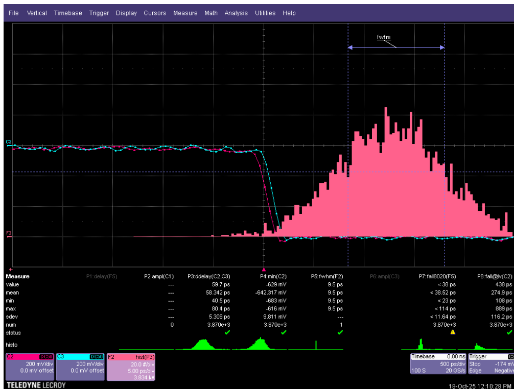
Figure 7. Experiment simulation using the external pico-second generator. Results: mean 58.342ps, sdev 5.309ps. DUT: LeCroy WP7300 3GHz 10-20GSa/s
