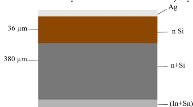
Figure 1. Geometric cross-section of the single-base photodiode structure Ag–nSi–n + Si–(In+Sn)
