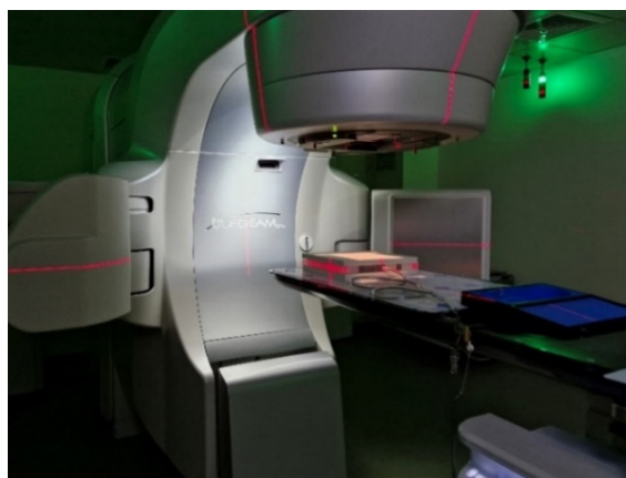
Figure 3. Photograph of measurement setup on TrueBeam with phantom and ionization chamber in position.
