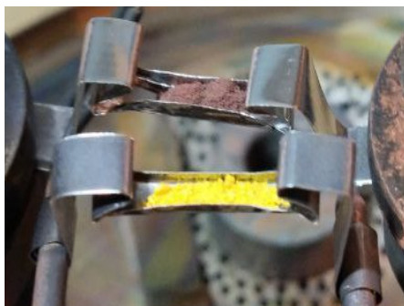
Figure 2. Photographic image of the BaS 3 and ZrS 2 in vacuum chamber
