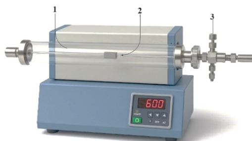
Figure 4. Schematic diagram of the device used for lithium diffusion: 1 – quartz tube, 2 – lithium sample, 3 – needle valve
