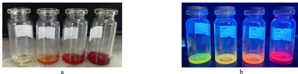
Figure 2. Photographs of CdTe QD samples at various reaction times, showing (a) solution color under ambient light and (b) photoluminescence under 365 nm UV light
