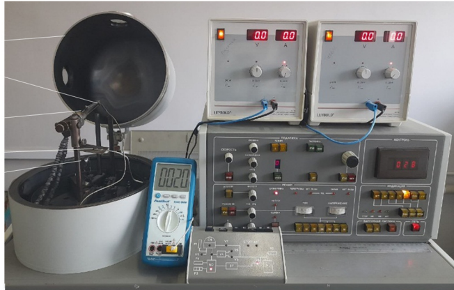
Figure 1. Schematic diagram of the vacuum chamber for obtaining \text{CdSe}_x\text{S}_{1-x} films 1-crucible (evaporator); 2-shield; 3-furnace and substrate; 4-thermocouple; 6-metal cover
