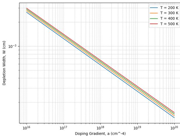
**Figure 2.** The width of the depletion region in a linearly graded p-n junction based on Si as a function of the doping gradient at different temperatures
