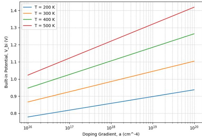
**Figure 5.** The built-in potential of a linearly graded p-n junction based on Si as a function of the doping gradient at different temperatures
