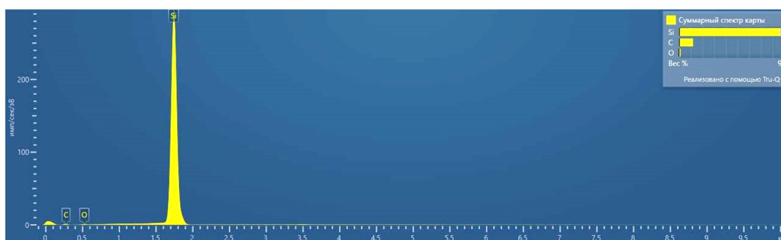
Figure 2. SEM spectrum of silicon doped with gadolinium during growth.
